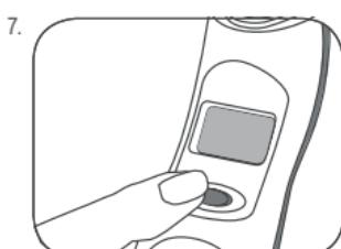
To power off, hold down the 'On/Mem' button for approximately 5 seconds, until the LCD screen shows 'o'. The thermometer will automatically shut down after 1 minute if it is however not turned off, helping prolong battery life.
