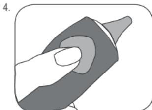
To measure the ear temperature, press the 'Scan' button until there is a long beep.
