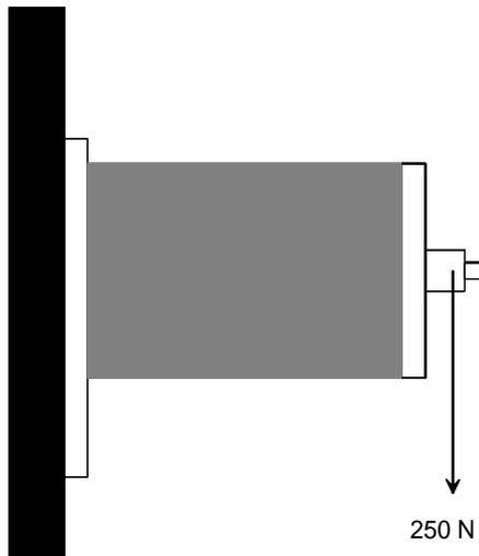
4.2.3. Apply a downward force of 250 N to the upper mounting plate. The resulting downward displacement should be recorded between 1 and 2 seconds after the onset of force application, and should be between 9 and 12 mm.
