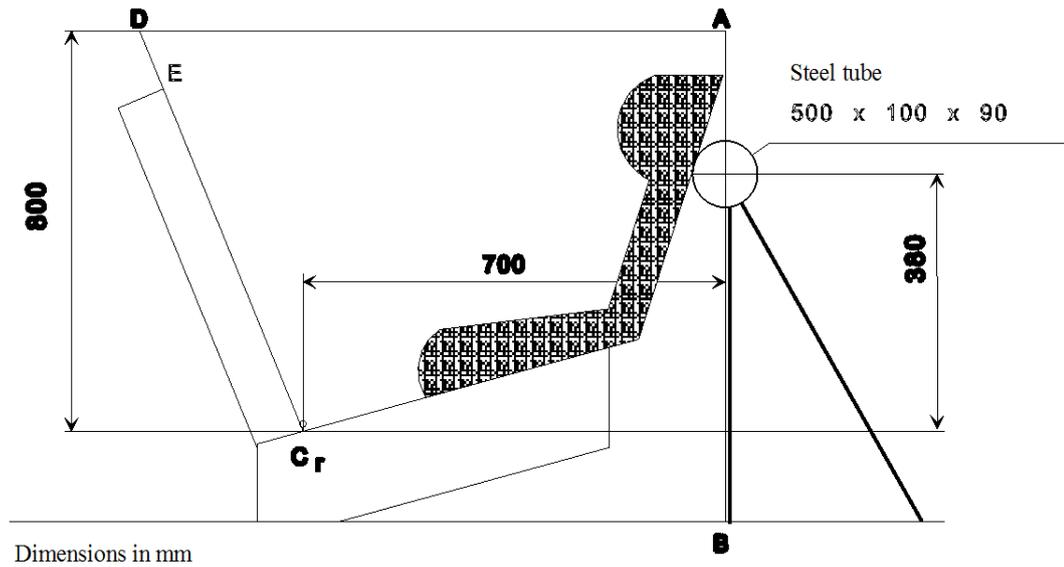
7.1.4.4.1.2.2. Child restraints in group 0 not supported by the dashboard, and carrycots: the head of the manikin shall not pass the planes AB, AD and DE as shown in Figure 3 below. This shall be judged up to 300 ms or the moment that the manikin has come to a definitive standstill whatever occurs first.
