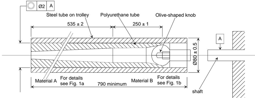
Play defined according to external diameter of polyurethane tube (light push fit)
